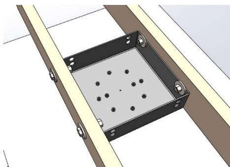
Bolt the ceiling bracket centrally over the hole. The bracket should rest on the plasterboard.
