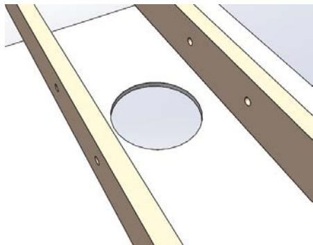
The fixing bracket is 350mm wide and can be bolted to the ceiling timbers. Frame out the ceiling, if required, to suit the bracket. Cut a hole in the ceiling plasterboard 240mm diameter.
