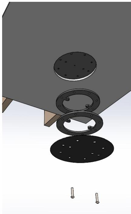
Bolt the spacers (as many as required), plus the ceiling cover into place. Use enough spacers so that the ceiling cover is almost touching the ceiling plasterboard. The ceiling cover should not clamp-up tightly to the plasterboard ceiling.
